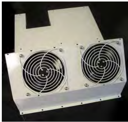
Figure 9 - Fan shroud removed from AnaSat ® transceiver
