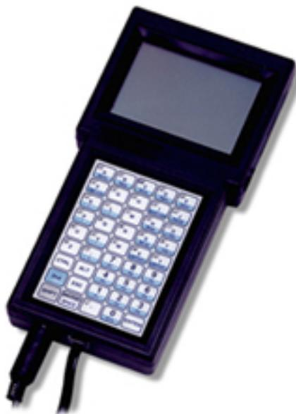
This document describes how to use the AnaCom Hand-Held Terminal (HHT) to monitor and control an AnaCom Transceiver (ODU) and AnaCom 1+1 Redundancy Systems. Hints on using other hand-held devices to monitor and control an ODU are provided as well.
