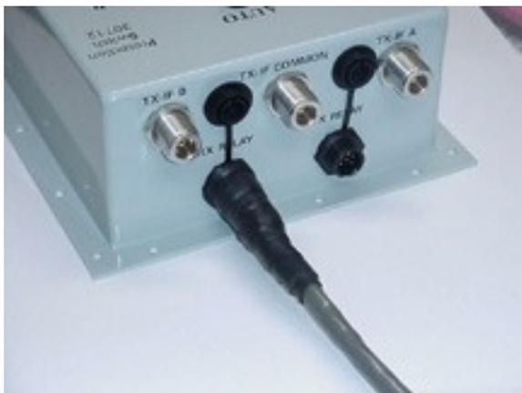
*Figure 2-2 Example of a properly weatherized connection*
