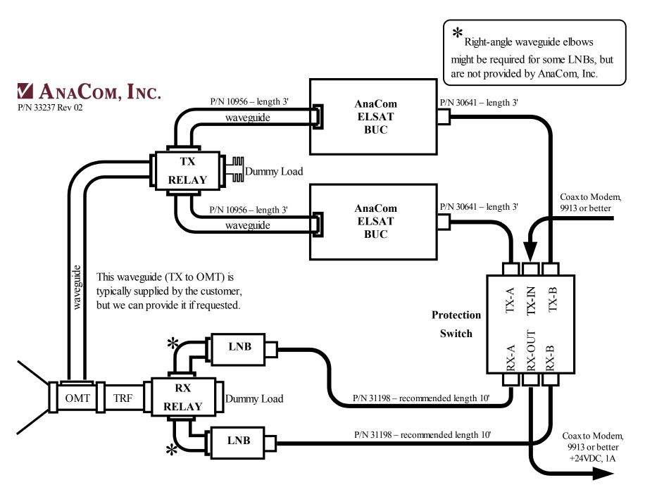
1+1 Redundant Protection Switch for two ELSAT BUCs and LNB protection. This diagram shows RF/IF connections only, the control cables (PS to BUCs & PX to Relays) are not shown
