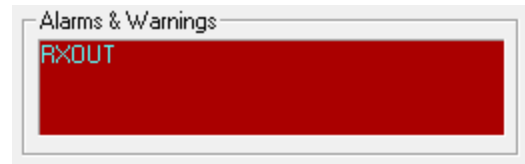
Example Alarm & Warnings panel in Supervisor 10's ODU Monitors window with a RXOUT error
