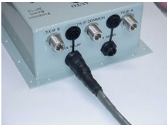
Figure 2-2 Example of a properly weatherized connection
